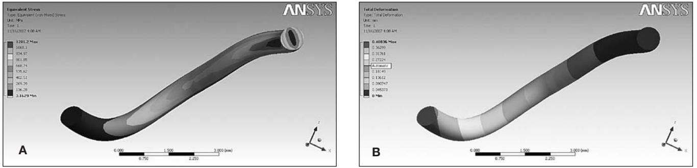
**Fig. 3 -** Stress distribution and displacements in the retainive arm of the round wrought wire clasp with a diameter of 0.7 mm: a. stress distribution, b. displacements.
