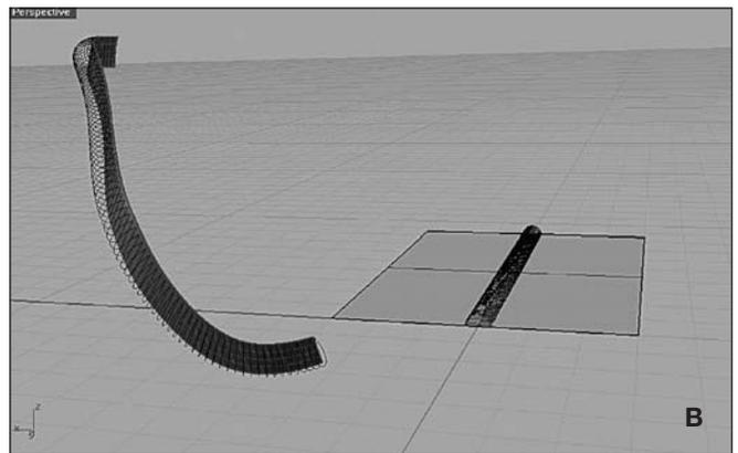
**Fig. 2** - 3D clasp modeling: a. round and b. half-round cross-section.
