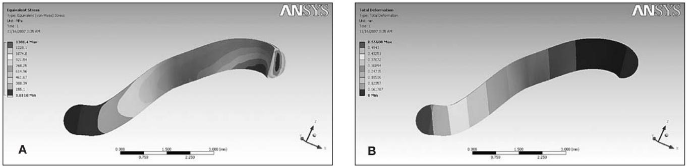
**Fig. 4 -** Stress distribution and displacements in the retainive arm of the half-round wrought wire clasp with a diameter of 1 mm: a. stress distribution, b. displacements.
